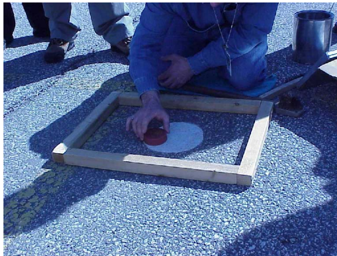
Photograph 2 Spreading the glass beads out into a “circle of beads” using a hockey puck
