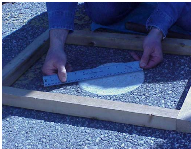
Photograph 3 Measuring the diameter of the circle of glass beads
