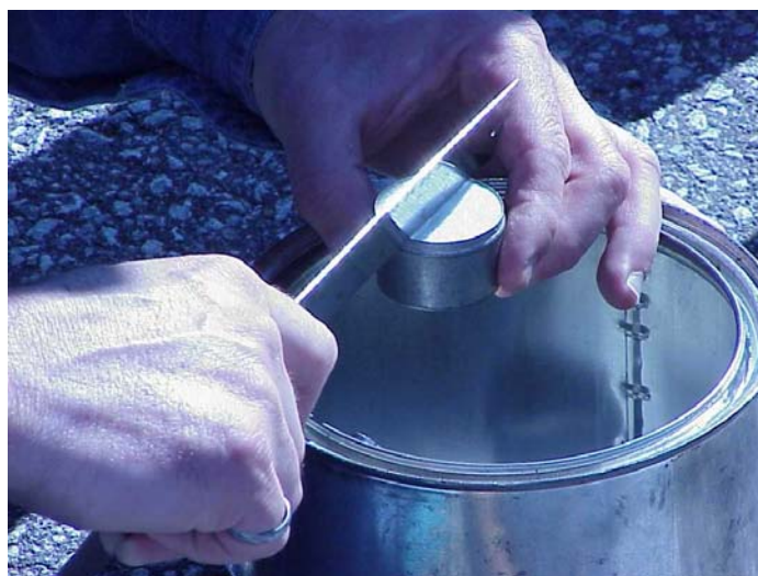
Photograph 1 Filling up an aluminum container with graded glass beads
