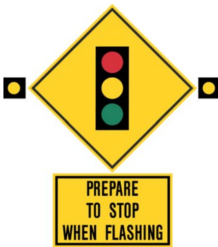
Figure 17 – Active Advance Warning Beacon
