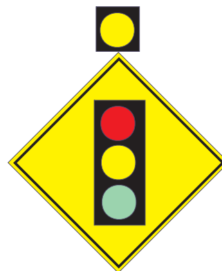
Figure 16 – Signalized Intersection Warning Beacon
