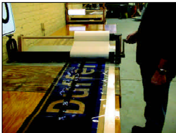
Figure 4.23 – Application of Transfer Tape to Reverse-cut Transparent Sheeting
