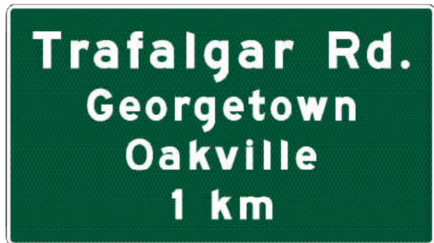
Figure 2.11 ADVANCE GUIDE Sign (Gf-1)
