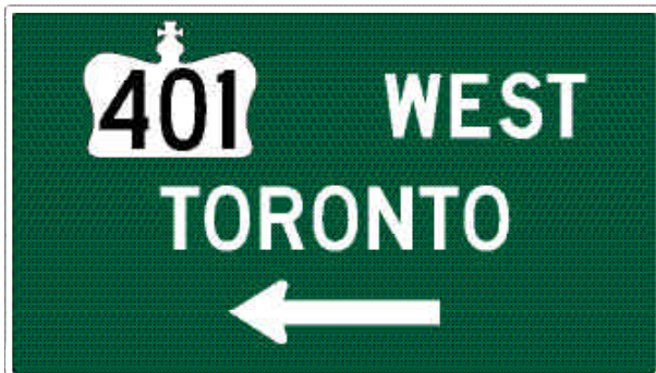
Figure 2.16 TURN OFF – LEFT TURN Sign (Gr-4)
