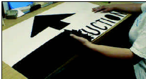
Figure 4.15 Transfer Tape Application to Sign Legend
